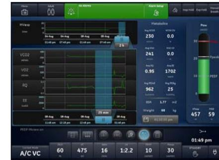
CARESCAPE Respiratory Module (optional) actually measures — not just estimates — VO<sub>2</sub> and VCO<sub>2</sub> and the ventilator software displays EE and RQ.
